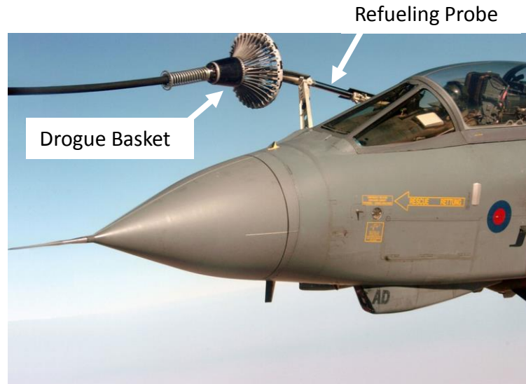
Tornado GR4 being refueling by a Probe-and-Drogue system
